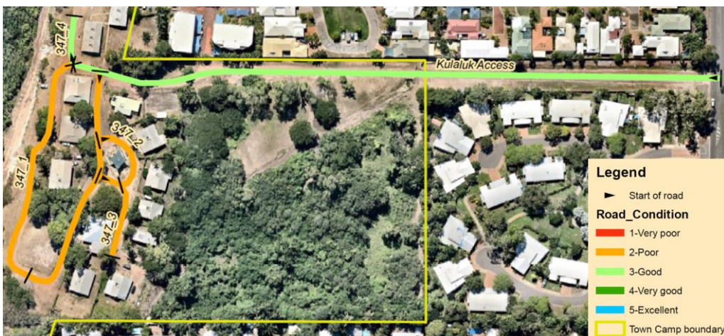
Figure 7 Road condition assessment
