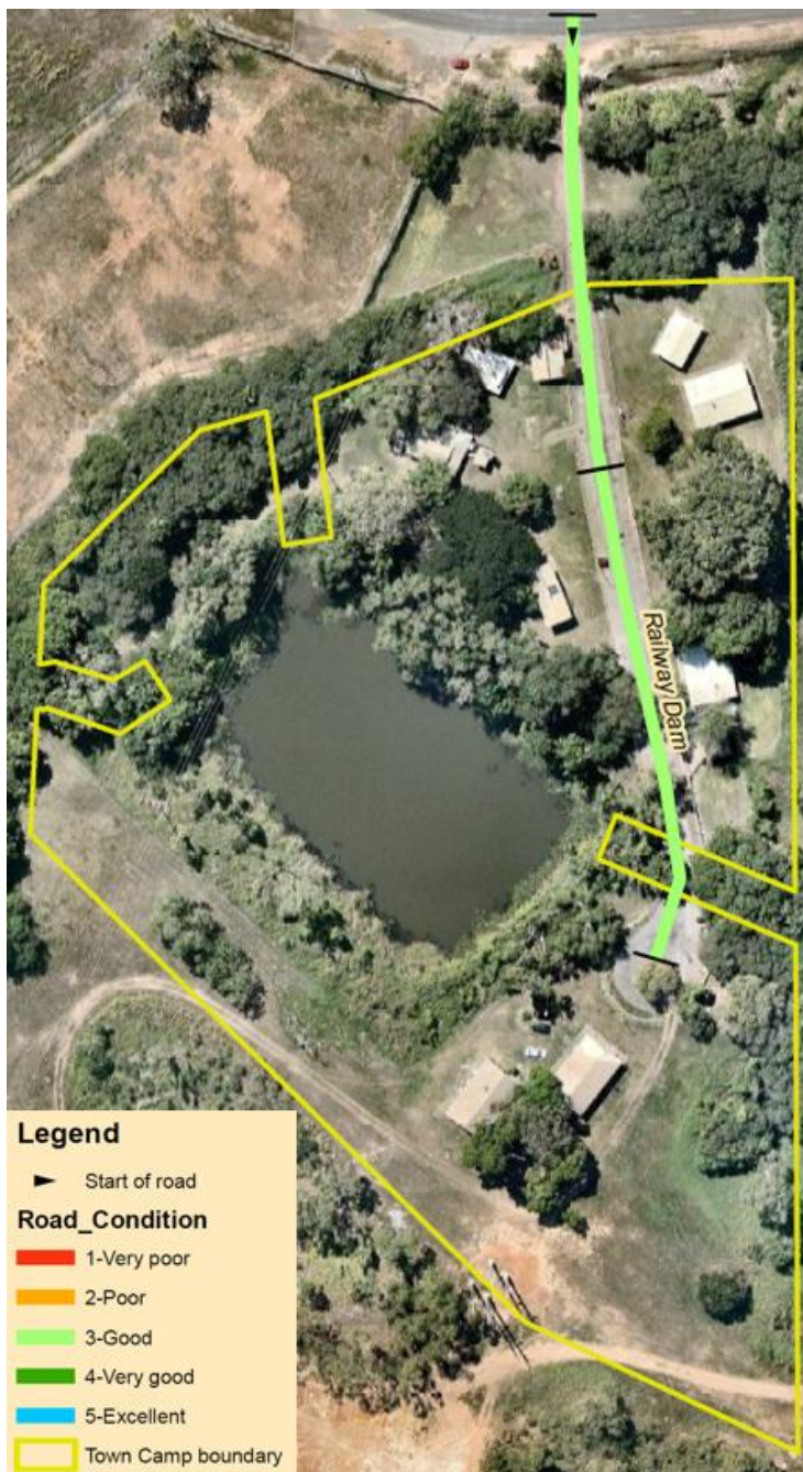
Figure 9 Railway Dam road network
