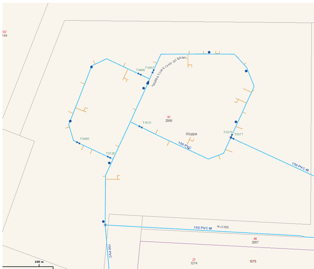
Figure 3 Wuppa water supply network
